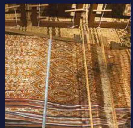
This Malay loom is set up with an intricate Ikat design in silk thread – the weft threads are dyed after the weft is set up on the loom.
