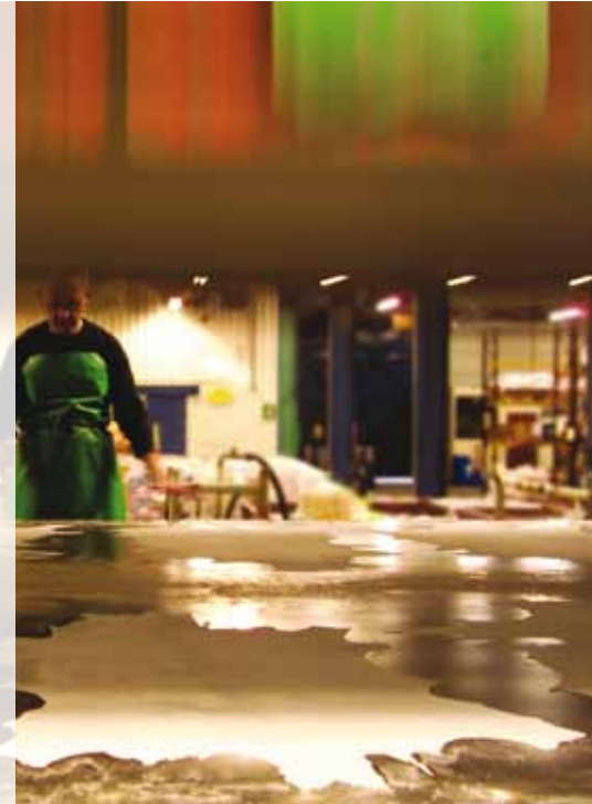
Vac drying: hides laid out and heated to 40°C Images courtesy of Pittards
