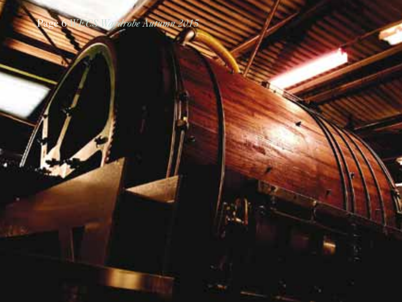
The Drum used to impregnate the skins with the dyes and other chemicals.
